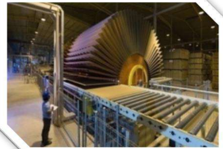
COOLING STACKING & HANDLING SYSTEM
