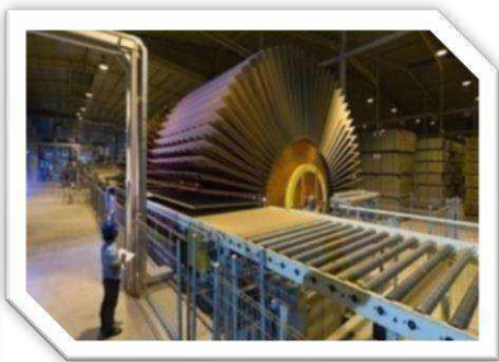
COOLING STACKING & HANDLING SYSTEM
