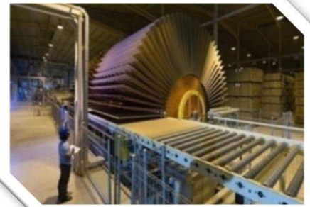
COOLING STACKING & HANDLING SYSTEM
