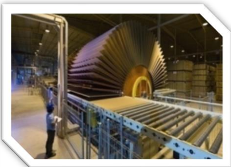
COOLING STACKING & HANDLING SYSTEM
